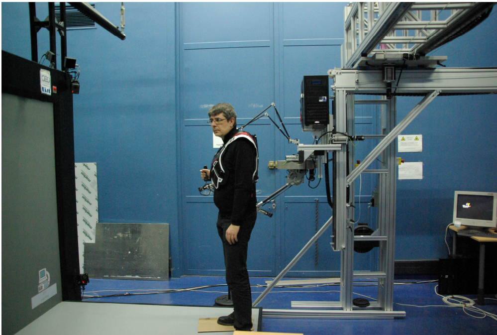
BOOM 3D in operation with one haptic device Virtuouse 6D35-45 (right side)
