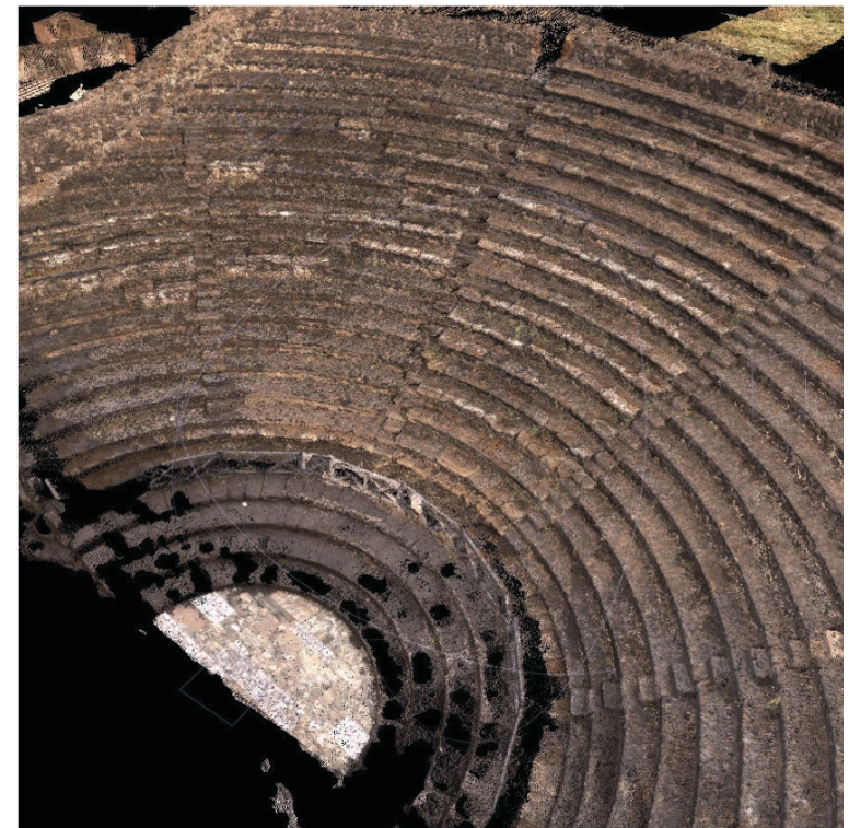
Fig. 7. The Odeon dense point cloud.
