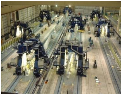
Airbus Automated Fastening Machines 165m long rail
