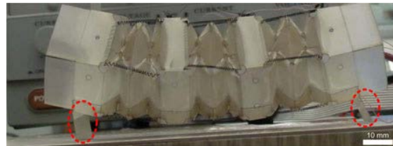
transformable worm robot
